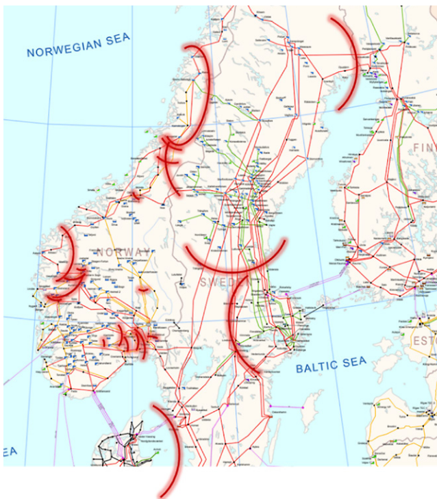
Figure 21: Approximate location of most restricting congestions in the simulation results. Swedish CNECs have been aggregated.
